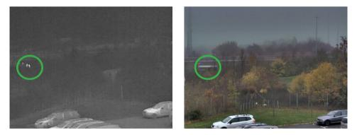
Figure 5. Images of persons taken with a thermal camera (left) and a visual camera (right) on a rainy day
