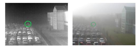
Figure 3 Image from a thermal camera (left) and a visual camera (right) on a misty day
